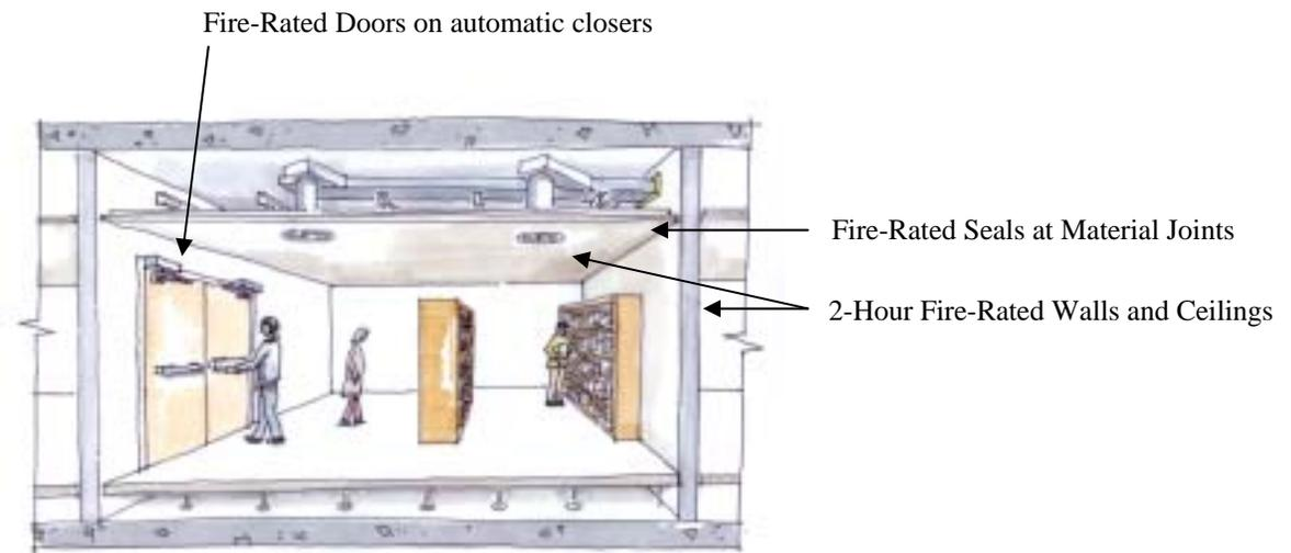
Figure 1. Special Collection Area separated through Compartmentation.
