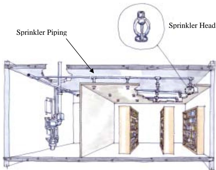
Figure 2. Typical Water Fire Protection System
