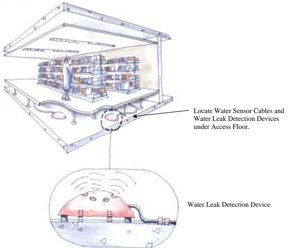
Figure 3. Water Leak Detection under Access Floors
