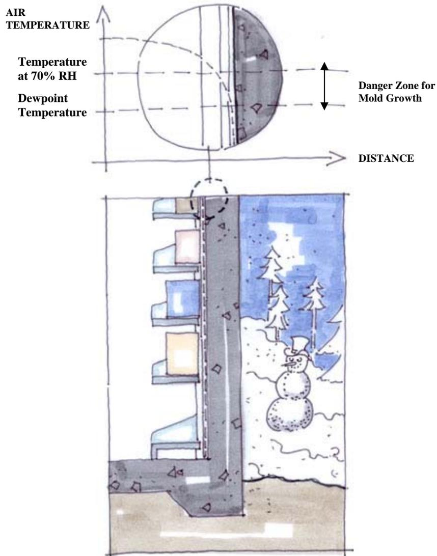
Figure 11. Microclimate of High Relative Humidity Against Exterior Walls
