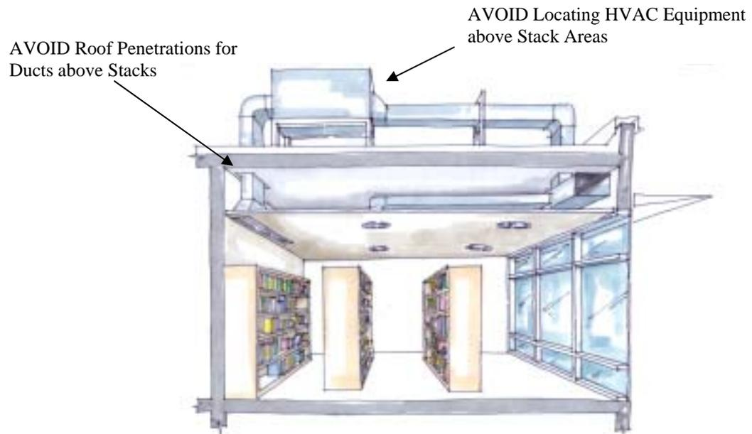
Figure 4. Illustration of Poor HVAC Equipment Siting.
