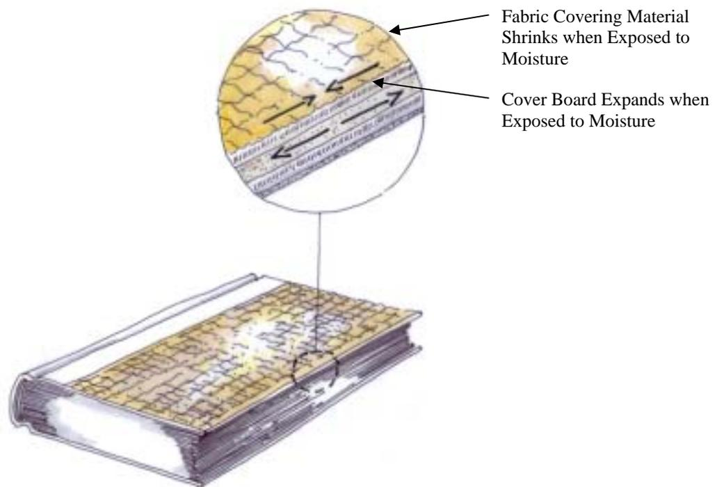
Figure 6. Different Rates of Expansion between Adhered Materials Produce Damage when Exposed to Moisture.
