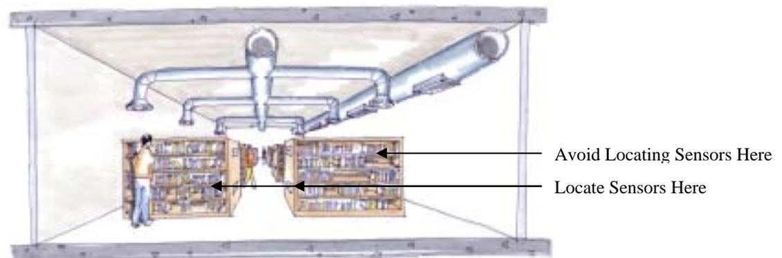
Figure 8. Place System Sensors away from Air Supply Outlets.
